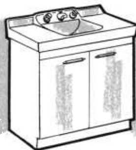
Lavatory-counter top set on cabinet.
