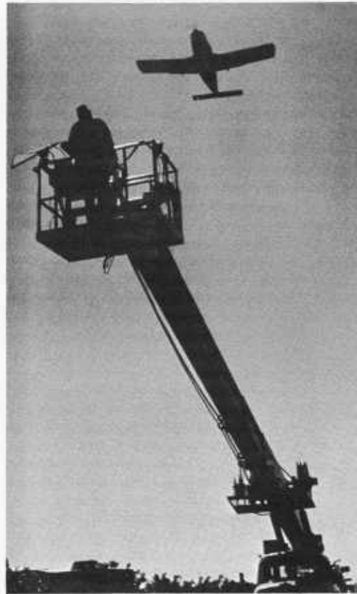
Infrared photos are taken from aircraft at USDA research station in Weslaco, Tex., with data from ground obtained simultaneously by use of a lift. "Ground truth" data correlate actual crop condition with aerial photos.
