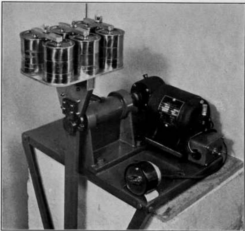
FIGURE 1.—Granulometer used for granulation tests.
