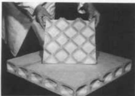
Spaceboard components are produced in two symmetrical halves, which are bonded together to form a three-dimensional structure.
