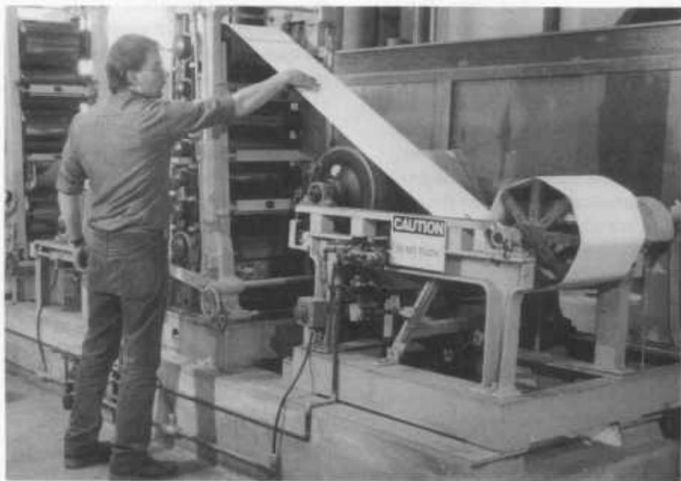
Paul Kmiecik, a physical science technician with the Forest Products Laboratory, checks the quality of recycled paper produced at the lab. Research focuses on altering the physical surface structure of pulp
