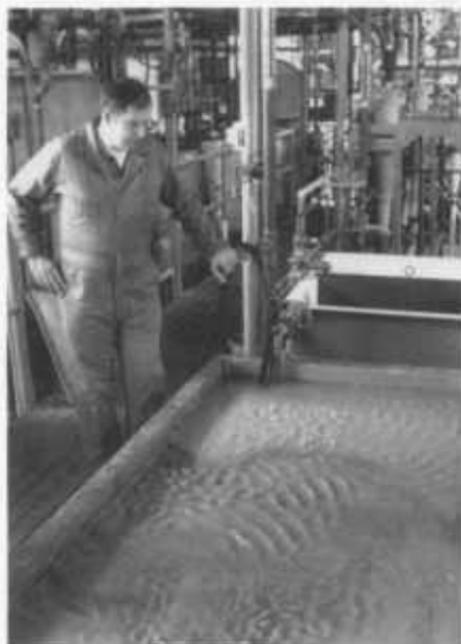
Dave Bromett, a chemical engineer with the Forest Service Forest Products Laboratory in Madison, WI, begins the process of separating oversized particles, lumps, and other contaminants, called "stickies," by passing the liquid paper pulp over a vibrating flat screen to produce usable fiber.
