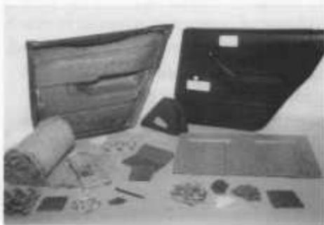
Recycled wood-based fiber and plastics can be used to produce a wide spectrum of products ranging from very inexpensive, low-performance composites to expensive, high-performance materials.
